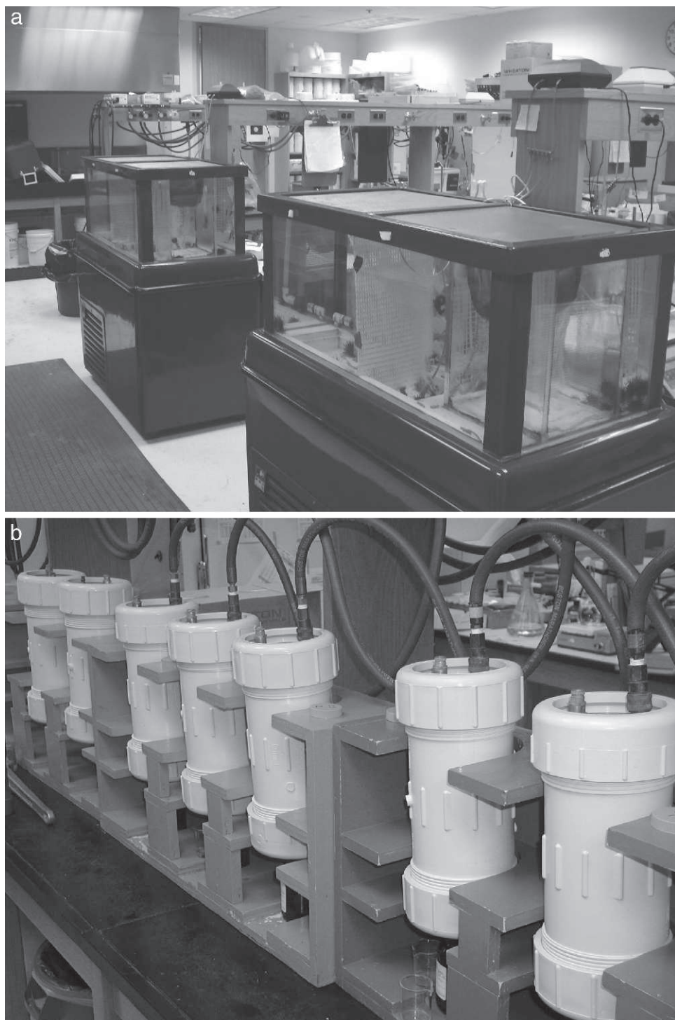
Fig. 5. Views of Ecotoxicology Laboratory utilized in Cooperative Agreement between CCS and USGS: (a) sea urchin maintenance tanks and (b) pneumatic porewater extraction devices (Photos by Marion Nipper).
